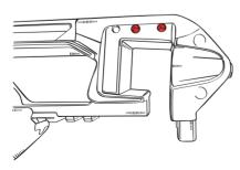
02: Align the String Stop with the rubber cap oriented towards the backend. Line up the holes of the String Stop with the corresponding screw holes above the limb pocket.
