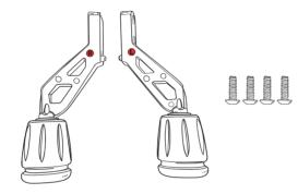
01: With the body of the crossbow laying flat on its side you will notice a set of screw holes above the limb pocket in the fore end of your crossbow. This where you will install the String Stops. The opposite side has another set of identical holes.
