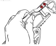
03: Attach the String Stop to the body of the crossbow using two screws (#10-24UNC 3/4").
